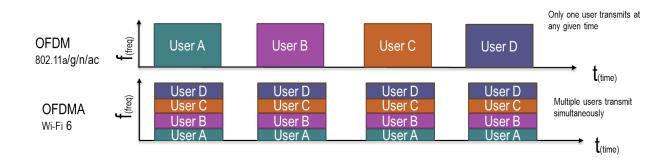
In the above example, 4 users, A, B, C and D, are transmitting simultaneously in the same OFDMA packet (i.e. time slot) thereby sharing the bandwidth of the channel. The maximum number of RUs per OFDMA packet is 37 in the 80 MHz band and 74 in the 160 MHz band.
