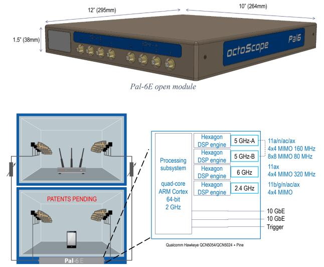
Pal-6E built into the smartBox; block diagram
