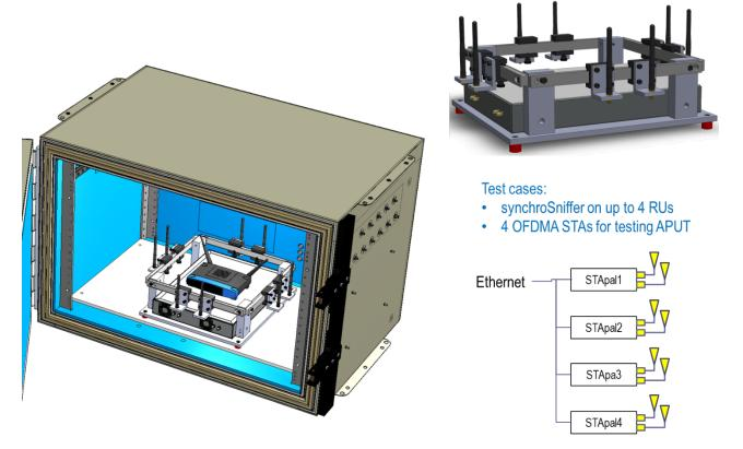
STApal open with the antenna system shown inside and outside of the octoBox chamber
