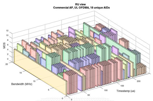
For OFDMA, since the RU/AID allocation changes from packet to packet, we need to show packet by packet plots. These packet by packet plots are called KPIs (key performance indicators) and are produced by dedicated synchroSniffer probes.
