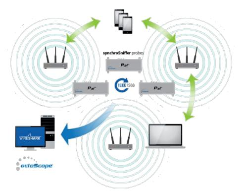
and DUT orientation. synchroSniffing is required for OFDMA – to simultaneously capture traffic on multiple AIDs (association IDs) that are assigned to different RUs (resource units).
