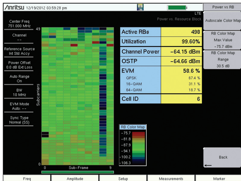
Figure 5. Power vs Resource Block (PvRB) is a critical measure of LTE modulation quality which shows the power level in each resource block as the subframes progress in time. The measurement shown here is made with the LMR Master's LTE Analyzer. Erratic or low PvRB can be caused by a number of factors including distortion in the channel cards or a fault in the power amplifier, filter, or antenna system. Such faults can lead to dropped calls, low data rate, low sector capacity, and blocked calls.
