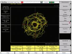
Demodulation – Error Vector Magnitude (EVM) This is the single most important signal quality measurement. Poor EVM leads to dropped calls, low data rate, low sector capacity, and blocked calls.
