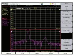
Distance Domain (DTF) analysis allows simultaneous viewing of cable return loss and distance to fault.
