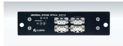
The single link Cubro Bypass for 1,10 & 100 Gbit single mode is realized with two MEMS optical switches. The switching mechanism offers the reliability of a solid state device. The optical switch is a latched version, this means it needs only power during switching operation. Even when power fails the optical switch stays in the programmed state.
