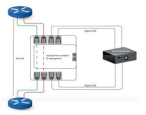
The illustration shows the general function of the optical switch device, and the switching path in the two modes. The device can also be used stand alone.
