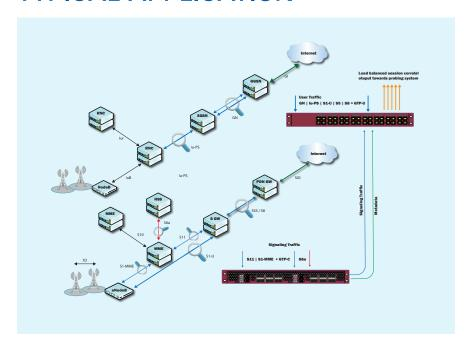
This is a typical application for EXA48600 and EXA24160 for GTP load balancing.
