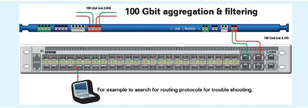
The Packetmaster EX48400 supports 4500 filters that can classify traffic based on layer 2 through 4 criteria. These filters can be used to redirect a selected part of the traffic to a low bandwidth monitoring tool, like a PC with Wireshark to trouble shoot an issue on a 100 Gbit link (such as a routing problem).
