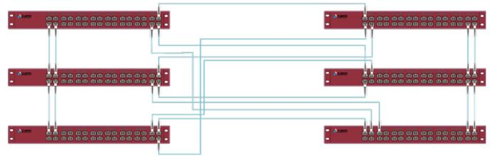
In this application 6 x EX32100 are connected to a fully meshed cross connect with 162 available 100 Gbps ports (27 per box). The interconnection between the boxes can be done with one link or more depending on the bandwidth that is needed.
