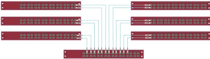
In this application 6 x EX32100 are connected to a central unit with 186 available 100 Gbps ports (31 per box).
