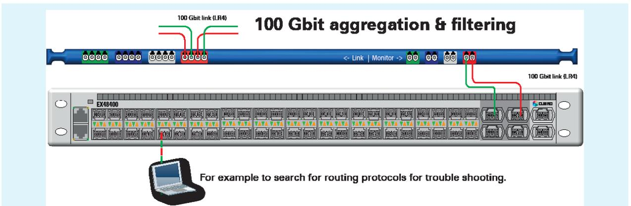
The Packetmaster EX32100 supports 8000 filters that can classify traffic. These filters can be used to redirect a selected part of the traffic to a low bandwidth monitoring tool, like a PC with Wireshark to trouble shoot an issue on a 100 Gbit link (such as a routing problem).
